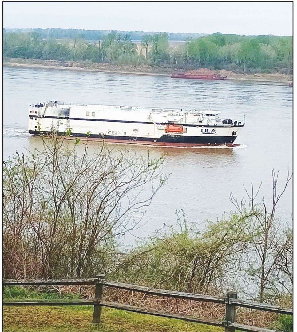
Lisa Knox took this photo of an unusual boat on the Mississippi River at Columbus one evening last week. The ULA website states "R/S RocketShip is a unique cargo ship used to transport rockets from United Launch Alliance's (ULA's) 1.6 million square foot production facility in Decatur, AL. RocketShip has been in use for nearly two decades, bringing Delta IV rocket stages to Cape Canaveral Space Force Station, FL, and Vandenberg Space Force Base, CA. In 2011, it started carrying Atlas V stages and now transports Vulcan stages. RocketShip is a highly maneuverable, unique custom-built rocket transport ship able to navigate both rivers and open ocean—the only U.S. flagged ship with this versatility. The roll-on, roll-off cargo ship is 312 feet long, weighs nearly 19 million pounds, has complete living quarters and dining area for its crew of 16, a heli-pad on the top deck, a below-deck machine shop and sophisticated computers and navigational aids on the bridge.
