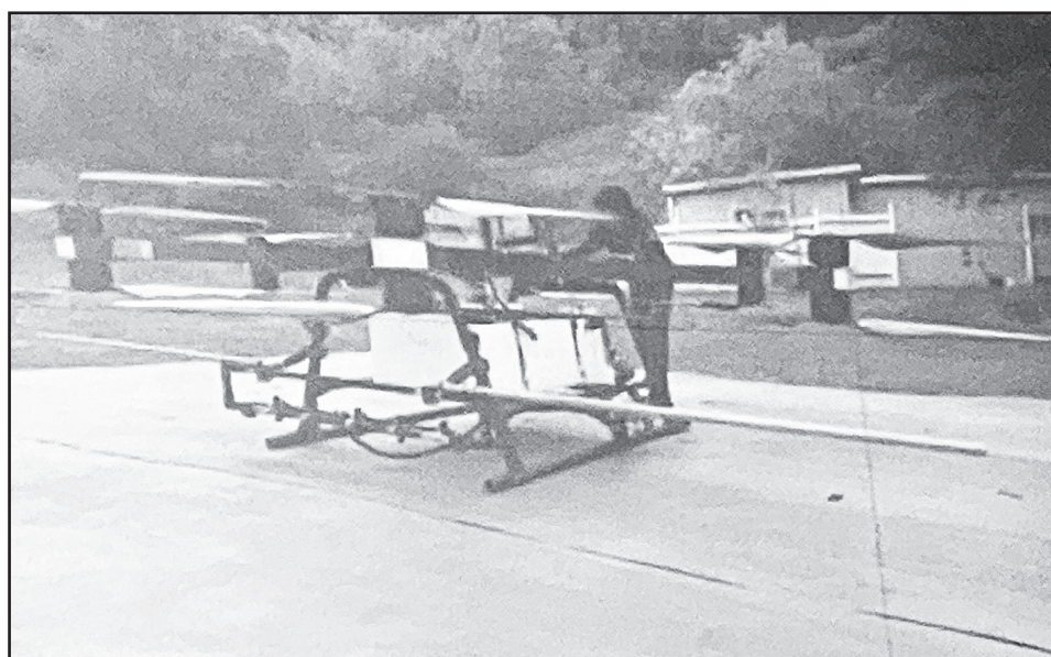
Alexis Scott with Spring Aerospace talked about a large-scale drone. Scott's presentation included a photo of a massive drone 12' L x 16' W; 6' L x 3' W (folded), with 70-gallon spray tank with collapsible boom.
