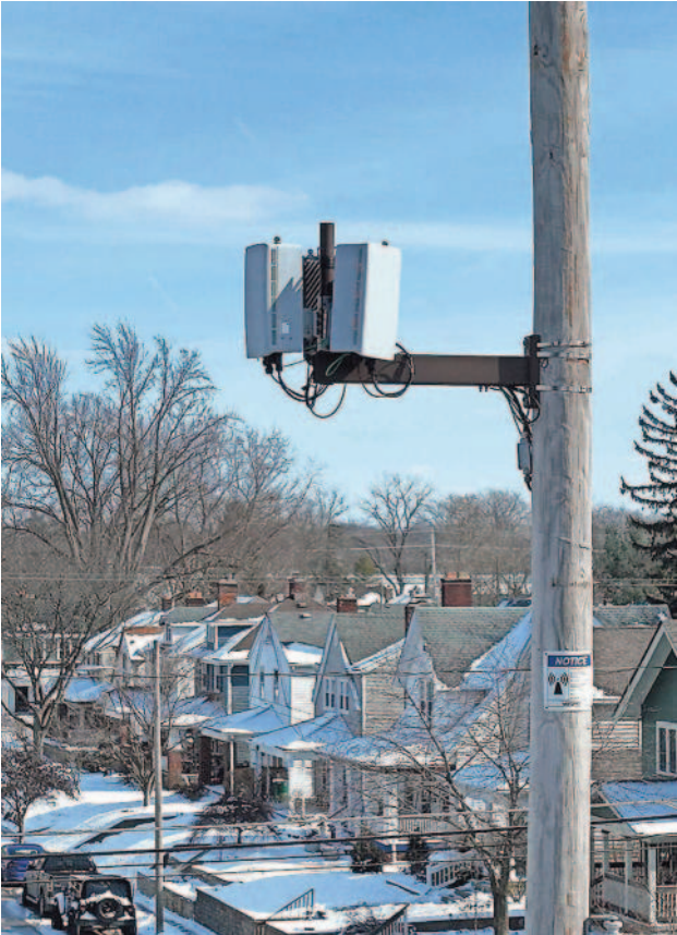
ShotSpotter gun detection equipment on a utility pole in Columbus’ Clintonville area.
