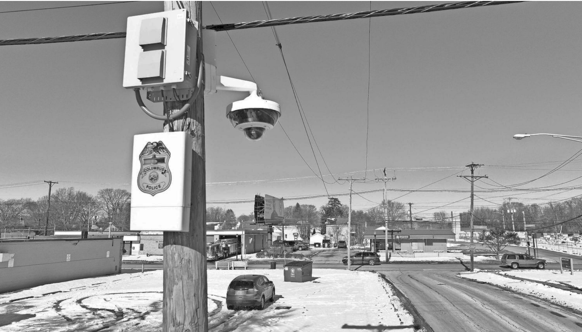
The ShotSpotter technology is used to pinpoint gunshots in high-crime neighborhoods including this area on E. Livingston Ave. The system alerts law enforcement when gunfire occurs. The system uses acoustic sensors to identify and locate the source of gunfire. DORAL CHENOWETH/COLUMBUS DISPATCH
