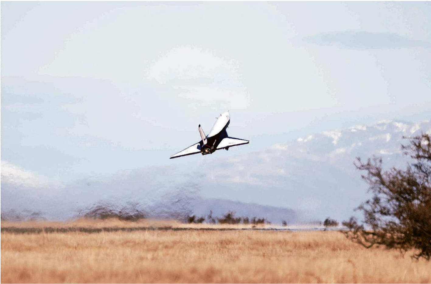
The Dawn Aerospace Mk-II Aurora spaceplane takes off during a flight test. Aurora is capable of reaching the edge of space and providing several minutes of microgravity for research payloads. PROVIDED BY DAWN AEROSPACE
